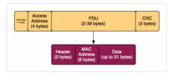
For advertisement communication channels, the access address is always 0x8E89BED6. For data channels, it is different for each connection.
